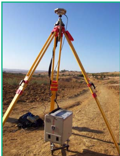
Every gravity survey must be carried out with a topographical survey. You can obtain the required elevation accuracy with a dual-frequency differential GPS survey without having to close your surveying loop. This is particularly useful in regional and local surveys. The caption above shows a GPS Leica system in action. A GPS base station is located less than 15 Km from the survey points. This base station is used for differential corrections either in real time or in post-processing
