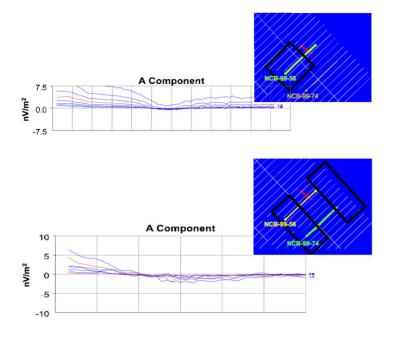
At 475 metres from the deposit (Hole NCB-99-74), the conventional **borehole EM survey** does not show any anomaly.
