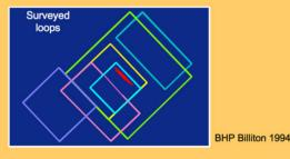
A conventional EM survey barely detects the deposit. Detection depends strongly on the loop location relative to the deposit.
