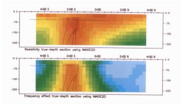
IP is an important tool for base metals exploration. Pseudosections converted through the algorithm of Image2D<sup>™</sup> clearly delineate the mineralized zone.
