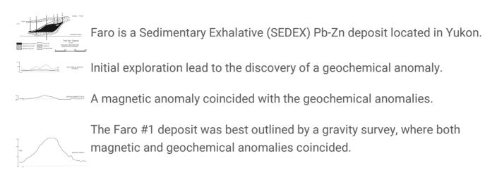
A 2.8 mGal anomaly coincided with the thickest section of the ore body.
