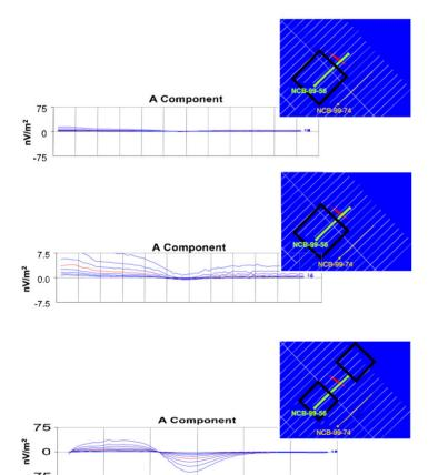
The Caber deposit (0.43 Mt @ 11.7 % Zn, 0.7 % Cu) is located in the Matagami mining camp. A conventional borehole EM survey and borehole InfiniTEM® surveys were tested at 200 metres and 475 m from the deposit.
