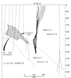
A borehole TDEM survey shows an off-hole response from sulphides located 150 metres west of the hole.
