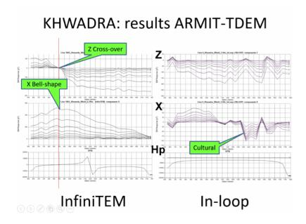
The InfiniTEM® loop configuration minimized coupling with the conductive overburden and revealed an anomaly associated with the massive sulphide lens, which the conventional inloop configuration could
