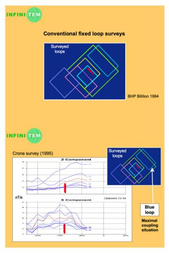
A conventional EM survey barely detects the deposit. Detection depends strongly on the loop location relative to the deposit.
