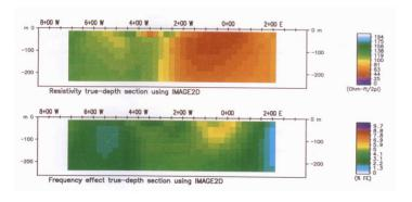
Conversion of the IP data with Abitibi Geophysics Image  $2D^{\mathsf{TM}}$  proprietary software localizes the deposit and shows that it has limited depth .
